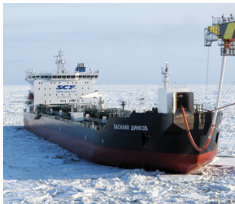
Vasily Dinkov, 70,000 tonnes (dwt) Arctic shuttle tanker, Barents Sea
